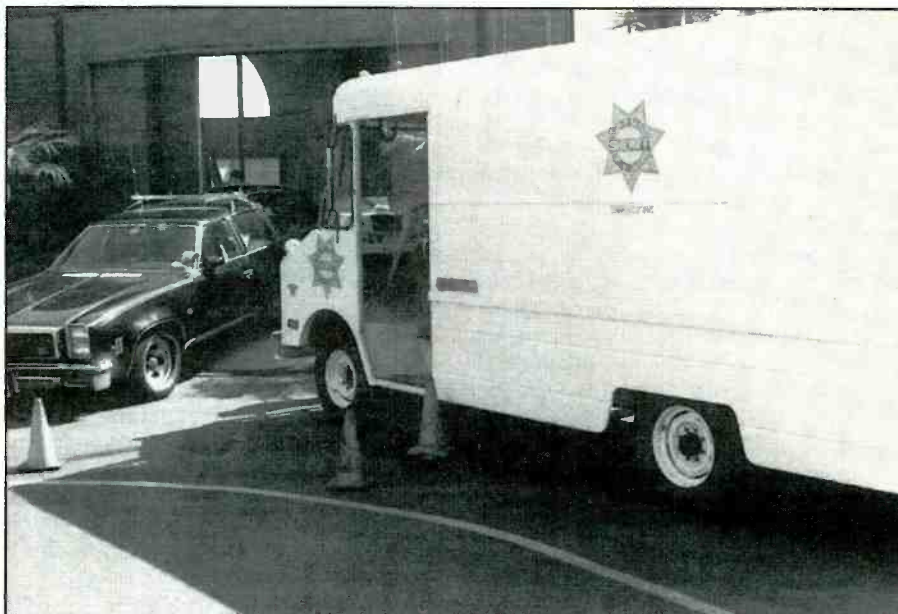
Close proximity of emergency vehicles may result in receiver desense problems. These two units are too close together.
