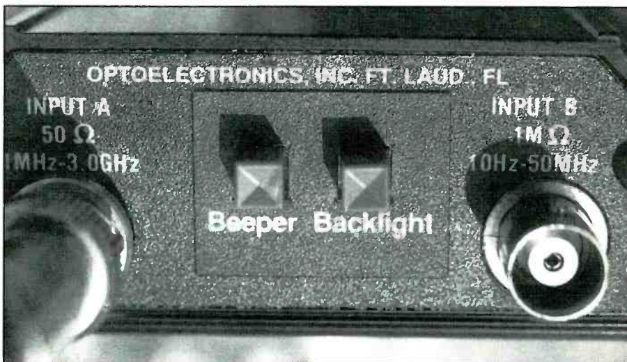
The optional "beep" function is a handy ALERT feature in the Optoelectronics frequency counter.
